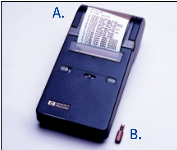
Detachable antenna unit shown mounted away from the control unit.
